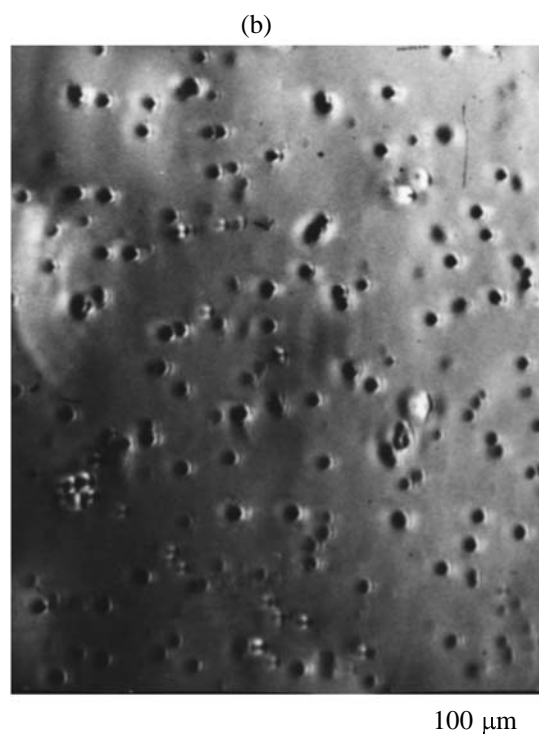
Fig. 4. Electron micrographs of elastomer films obtained from B-160 latex and modified with silver particles. Residual moisture content, %: (a) 15 and (b) 5.
